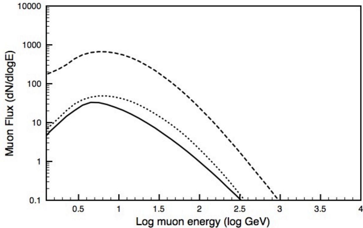
Enhanced muon flux in case 1 (dots) and case 2 (dashes) compared with the normal muon flux (solid).
