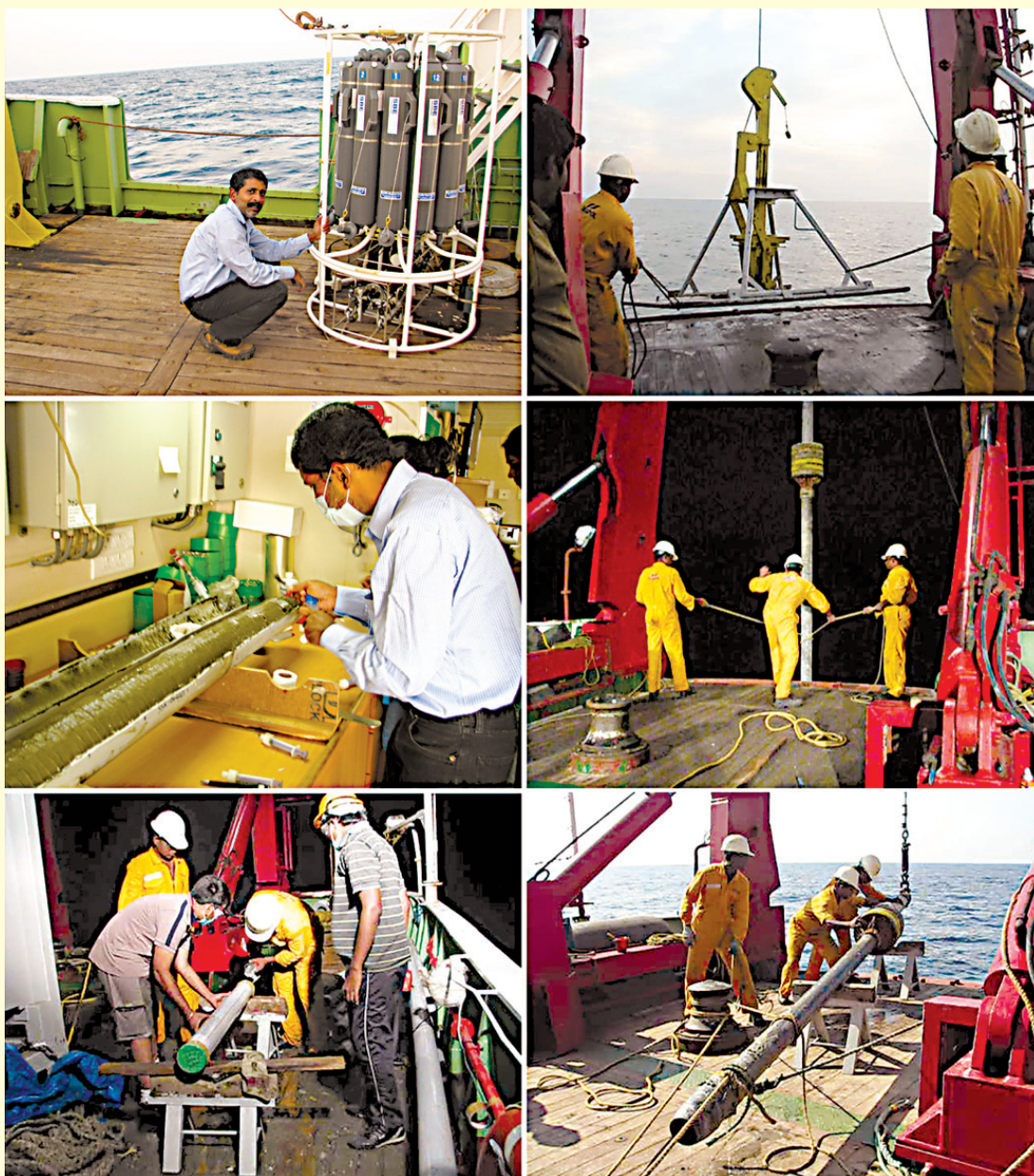
Major activities during the research cruise SSK042 onboard CRV Sindhu Sankalp (CSIR-NIO). Clockwise from top left: CTD profiling and water column collection; spade coring operation; gravity core deployment; gravity core recovery; cutting of three meter long cores into two D-halves; sampling and analysis along the length of the sediment cores.
