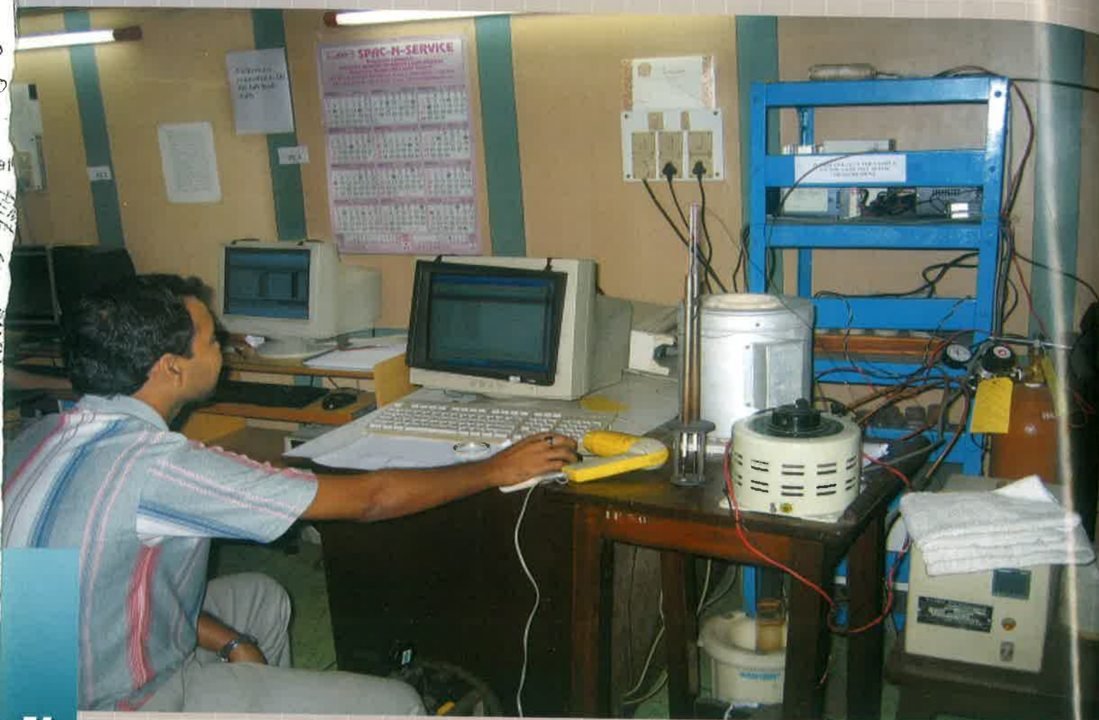
Ac-Impedance analyzer with low and high temperature setup
