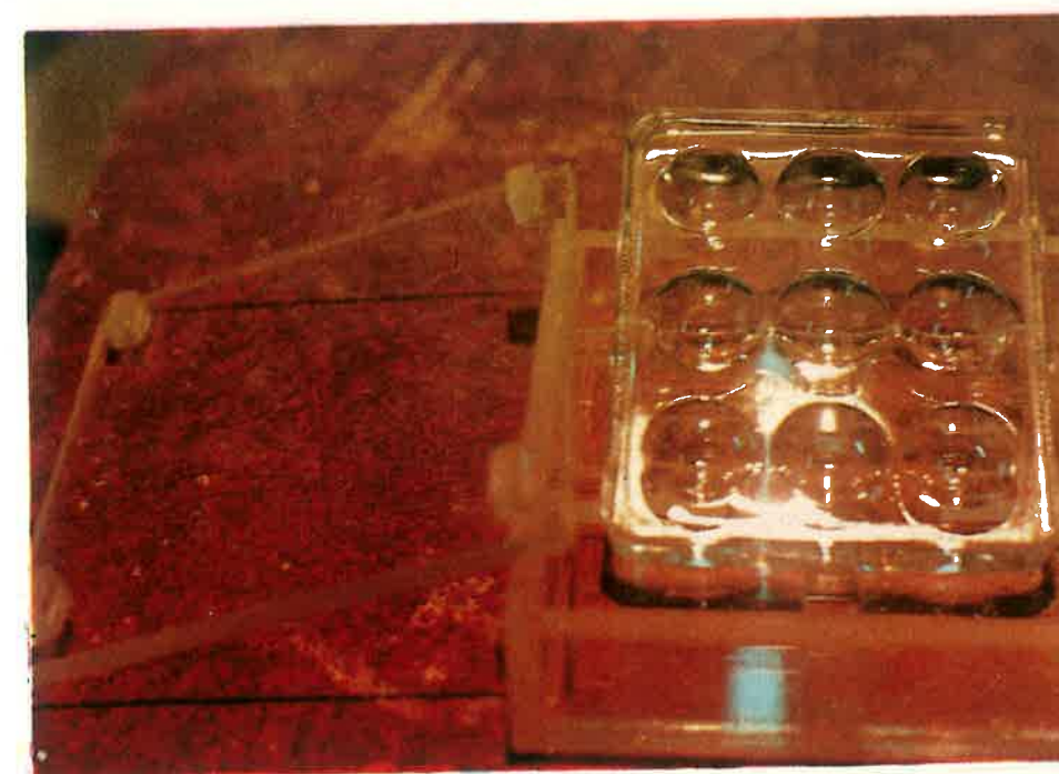
A plexiglass box designed by Dr. R. Chattopadhyaya for macromolecular crystallization, manufactured at the Bose Institute Workshop
